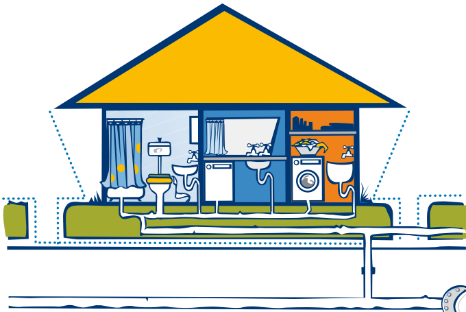
House wastewater pipes
